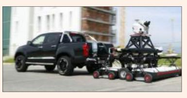
and a Stream EM GPR array for below-ground objects.
