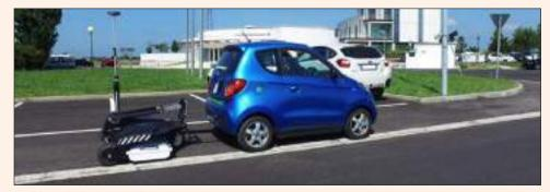
Hexagon's IDS GeoRadar division has also just introduced the Stream C, a compact GPR array solution for real-time 3D mapping of underground utilities. This solution comes equipped with software for automatically mapping
